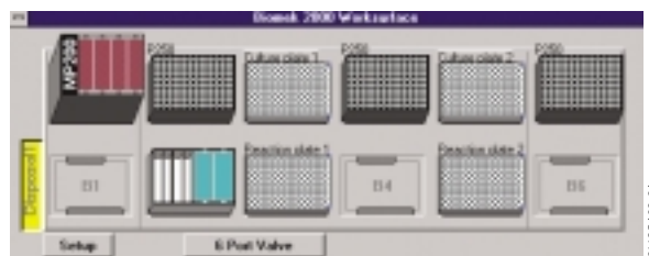
Figure 3. Deck configuration of the Biomek® 2000 for the CytoTox 96® Non-Radioactive Cytotoxicity Assay (Cat.# G1780). The only tool needed is the MP200 tool positioned at A1. Positions B1, B4 and B6 remain empty. P250 tip boxes are placed at positions A2, A4 and A6. Position B2 holds a reservoir that contains 8ml of Nuclease-Free Water (Cat.# P1193), 12ml of CytoTox 96® Substrate and 12ml of CytoTox 96® Stop Solution. The 96-well culture plates containing the ACTIVTox® cells are placed at positions A3 and A5. Two empty, flat-bottom 96-well plates are placed at positions B3 and B5.
