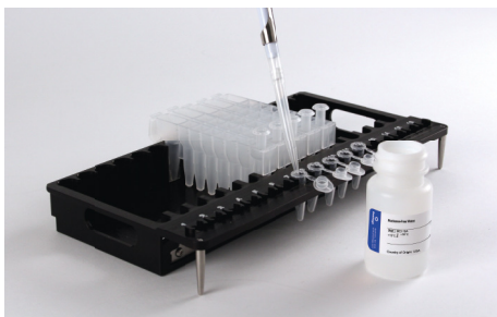
Figure 1. Maxwell® RSC Cartridge. Cultured cell sample is added to well #1, and a plunger is added to well #8.
